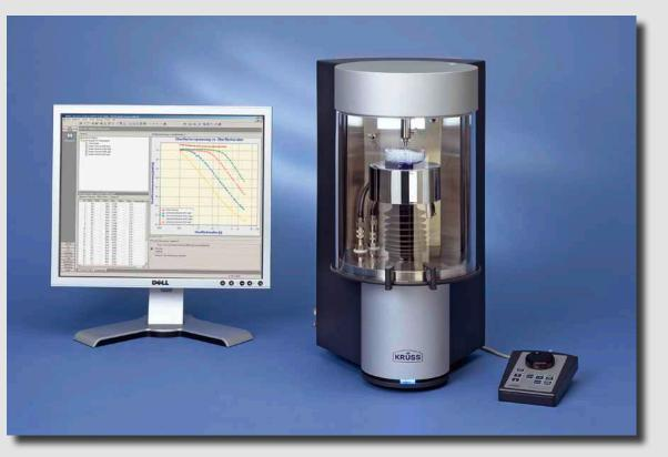
*Printing – bonding – spraying – cleaning*: processes such as these require surfactants that are already effective in fractions of a second – and an instrument that can record their effectiveness. The Bubble Pressure Tensiometer BP100 determines the dynamic surface tension as a function of the surface age. Thus the instrument provides information about wetting and drop formation in rapid processes.
