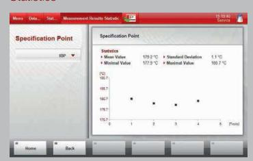
The ADU 5 software features a well-arranged overview of all relevant statistical data. The statistics program automatically calculates the mean, max and min value and the standard deviation for selected samples. You can choose between different specification points:
